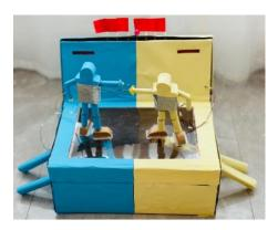
Magnetic Fencing was inspired by Tristen's love for watching fencing matches during the Olympics. Magnetic control sticks are used to manoeuvre the fighters. An electronic system detects when the sword of a fighter touches the body of its opponent, and this triggers a motor that activates the health bar as well as a buzzer and light bulb.
